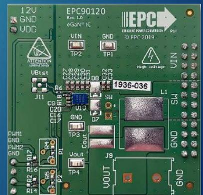
*EPC90120: 80 V Half-bridge with Gate Drive, Using EPC2152*
